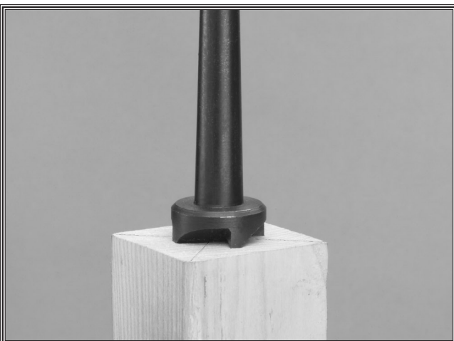
Figure 25. Spur center properly embedded into workpiece.
